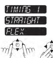
**Set Timing Mode** Use the left and/or right arrow keys to choose Straight, Flex or SENSITIVITY. Press the P key.
