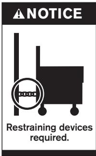
2. The restraint means must be attached to the rear of the Keating Gas Fryer within 2" of the center line width and approximately 1-5/8" from the bottom of the cabinet back to allow the restraining bolt to be anchored to the cabinet back between the cabinet bottom and inner liner.
