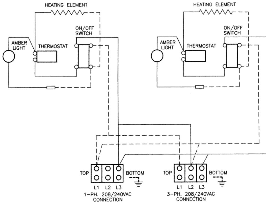
**36" WIDE ELECTRIC GRIDDLE WIRING DIAGRAM**
