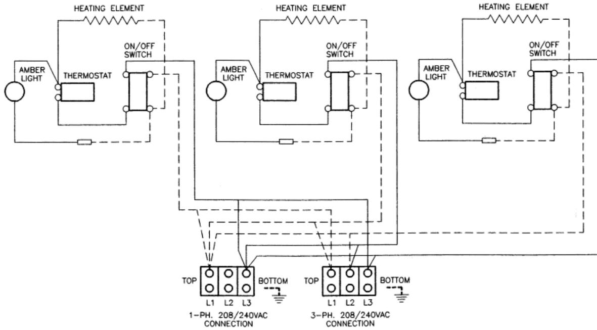
**42" - 48" WIDE ELECTRIC GRIDDLE WIRING DIAGRAM**
