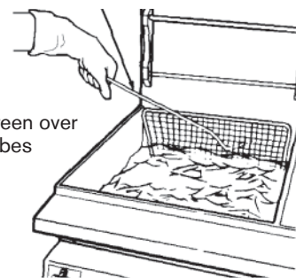
DRAIN CLEAN OUT ROD
