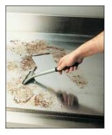
Scrape the griddle with the Keating scraper with replaceable blades.
