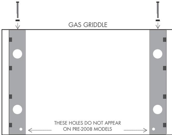
4. On Gas Griddles, add a 1/4"-20 x 3/4" Hex Screw (part # 032328) through the front edge of the cabinet bottom and leg channel. The holes for this exist and will be inline if the leg channel is installed properly. Secure with 1/4"-20 Serrated Flange Nut (part # 031567).
