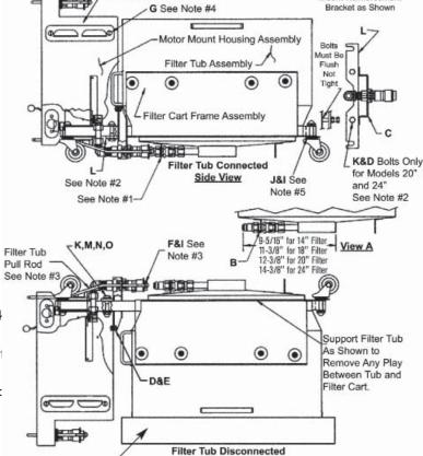
3. Attach filter tub pull rod handle using Items F and I.
