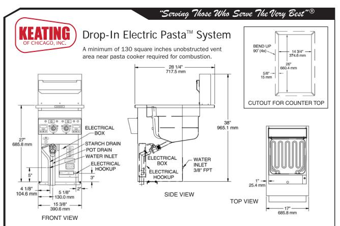
Description - The Keating Drop-In Pasta™ System can be ordered in electric 208-240 Voltage in single or three phase.
