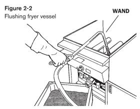
6. Repeat this procedure as necessary until fryer vessel is completely flushed out. Partially close drain valve to permit fryer vessel to fill above tubes/elements permitting swirling action to rinse down fryer vessel.
