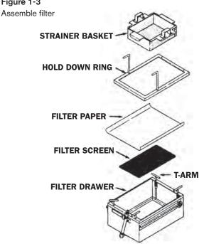
NOTE: Hold down ring makes a gasket-like seal on filter paper. Filter paper must be placed edge to edge from front to back, overlapping on sides. Filter Paper must be smooth and flat under hold down ring to get a proper seal. Lock the two tension arms into place by pushing down and rotating 90°.
