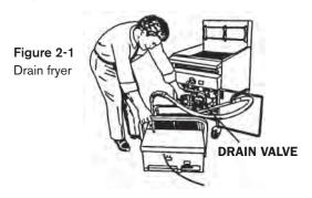
3. Open fryer cabinet door and position portable filter vessel under fryer drain valve. Slowly open drain valve to avoid splashing and permit oil in fryer vessel to drain into filter vessel (Figure 2-1).
