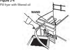
10. Operate pump for approximately thirty seconds after filter vessel is empty to clear any residual oil from the filter's lines/hoses. This will prevent blockage resulting from solidified oil during subsequent filtering operations.
