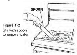
3. Use the spoon and stir oil thoroughly until bubbling stops, resulting in removal of all water (Figure 1-2).
